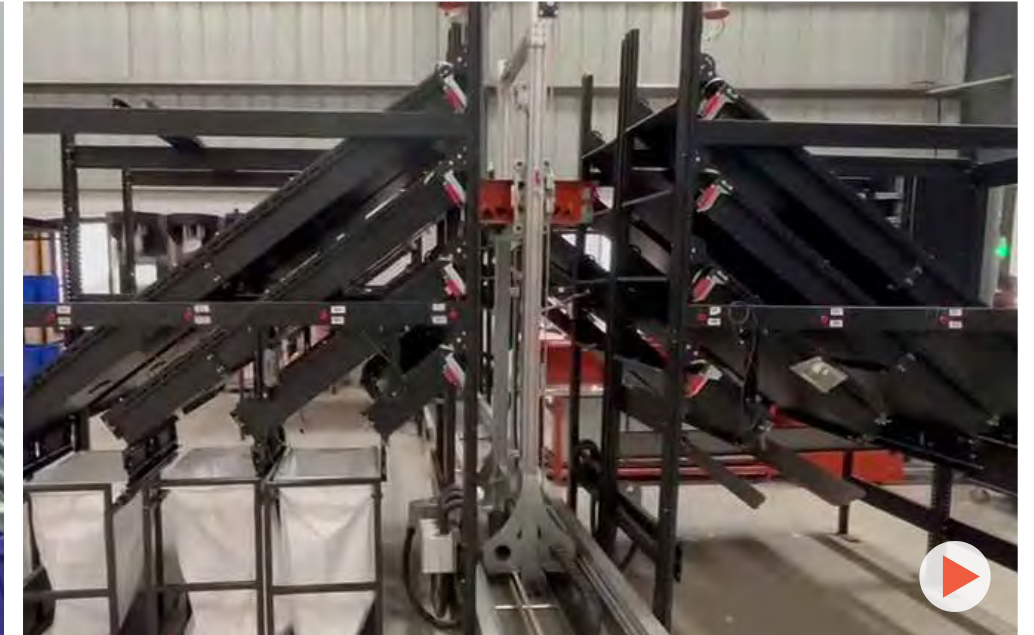
Astro Sort V | Vertical sortation of items to chutes | Industry: Courier express parcel/ 3PL
