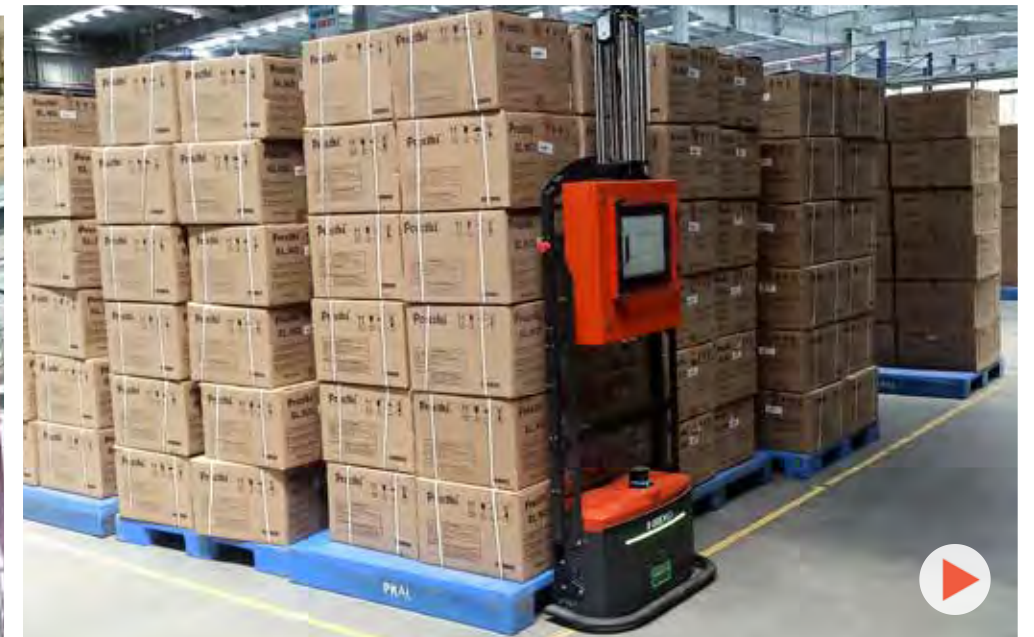
Pallet handling autonomous mobile robot | Unmanned movement of palletized loads | Industry: Appliances
