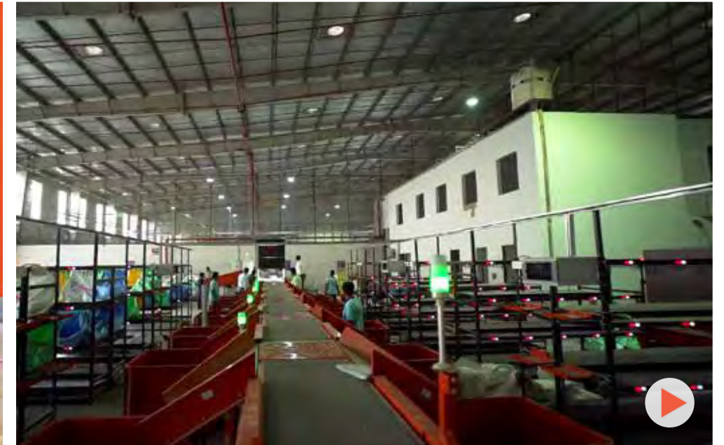
Steerable wheel sorter, PTL system, Carriage belt sorter | Scanning, weighing, dimensioning and sorting | Industry: Courier express parcel
