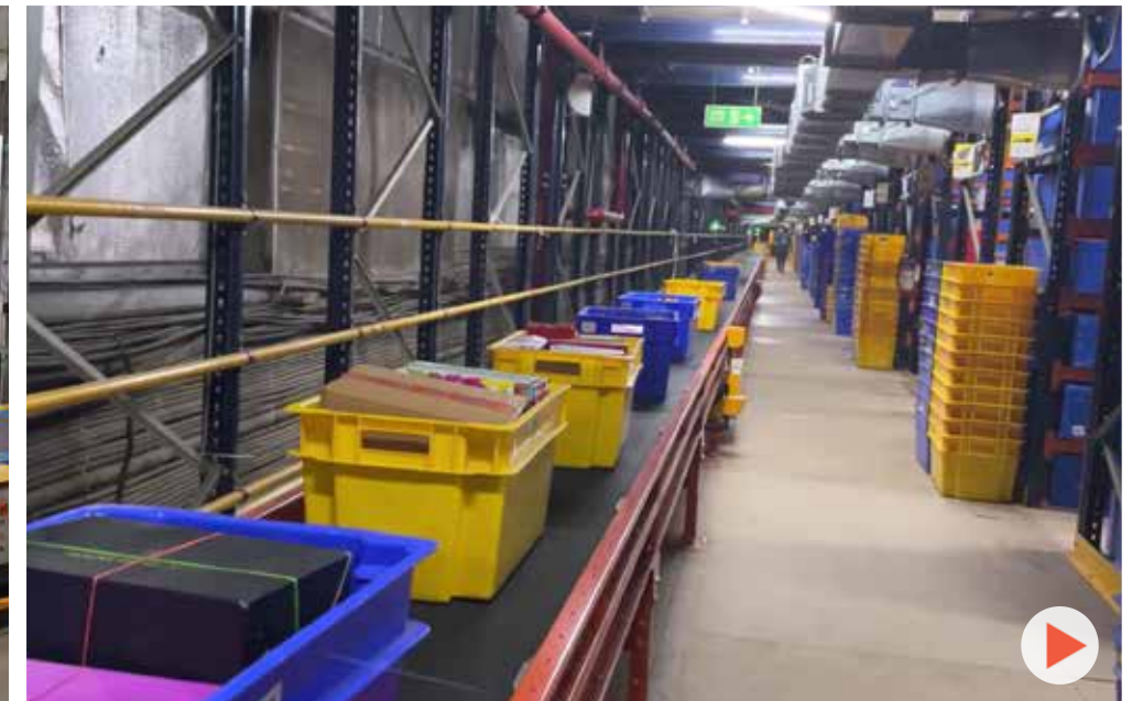
Solution: Tote handling and sorting | Conveying, colour based sorting, traffic management | Industry: E-commerce
