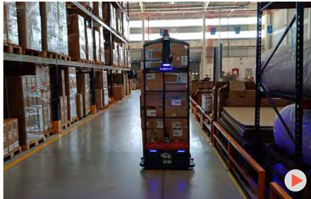
Solution: Pallet handling autonomous mobile robot | Unmanned material handling with pallet management application | Industry: Sports retail
