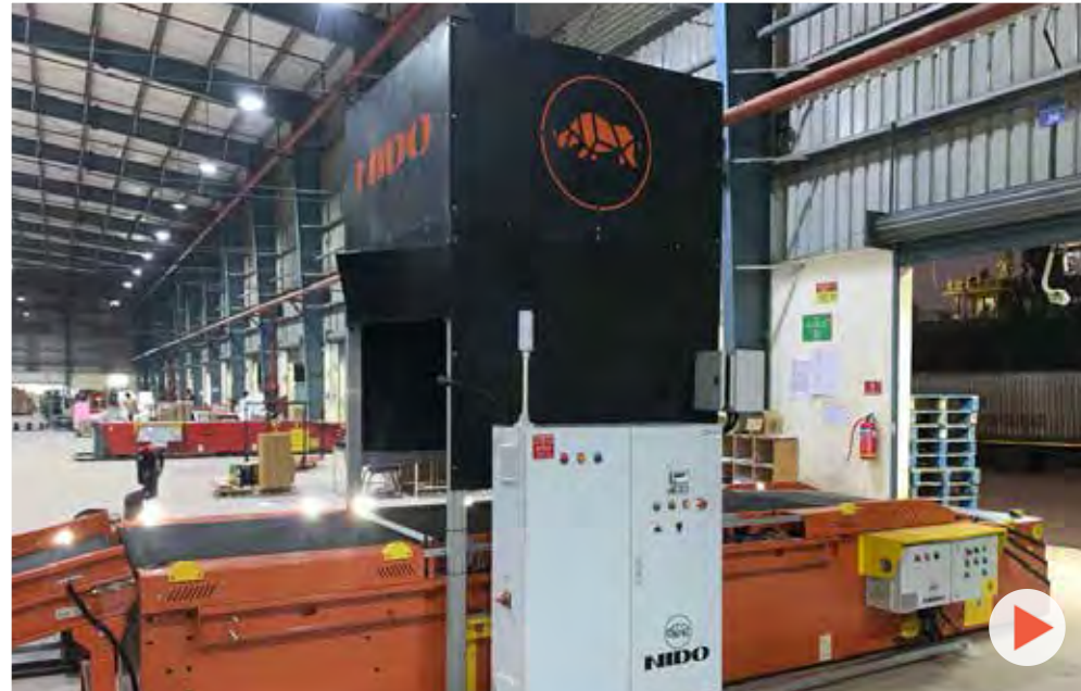
Telescopic belt conveyor with dimensioning and weighing Loading and unloading, scanning, weighing and dimensioning | Industry: 3PL
