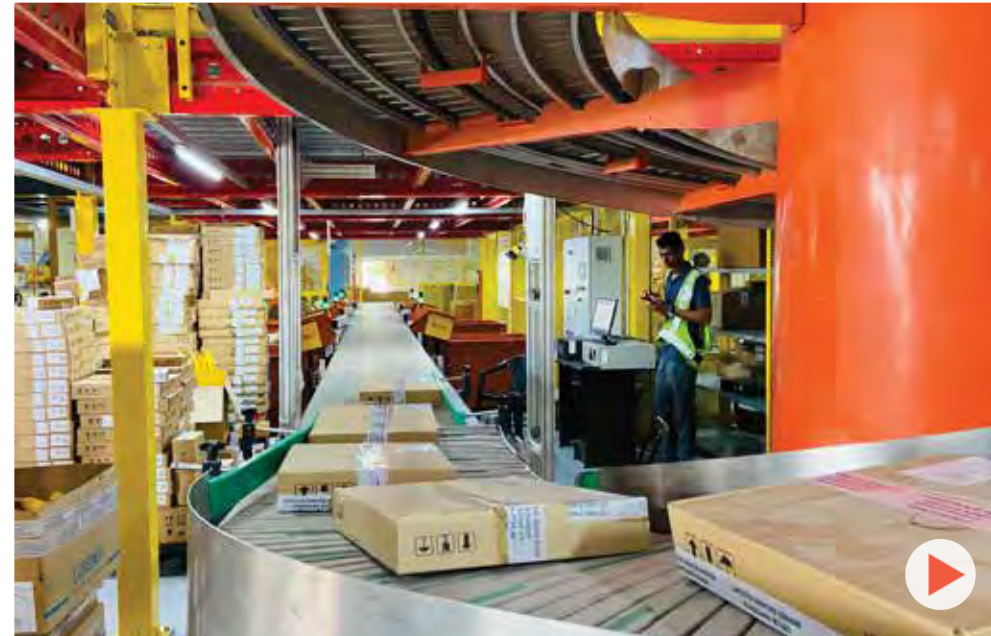
Motorized spiral conveyor, linear arm sorter | Vertical transport and sorting | Industry: Courier express parcel
