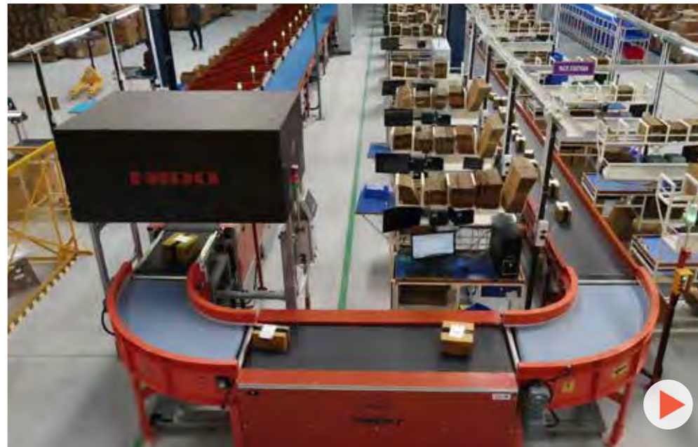
Conveyor, DWS system, Linear arm sorter | Scanning, weighing, dimensioning and sorting | Industry: Cosmetics
