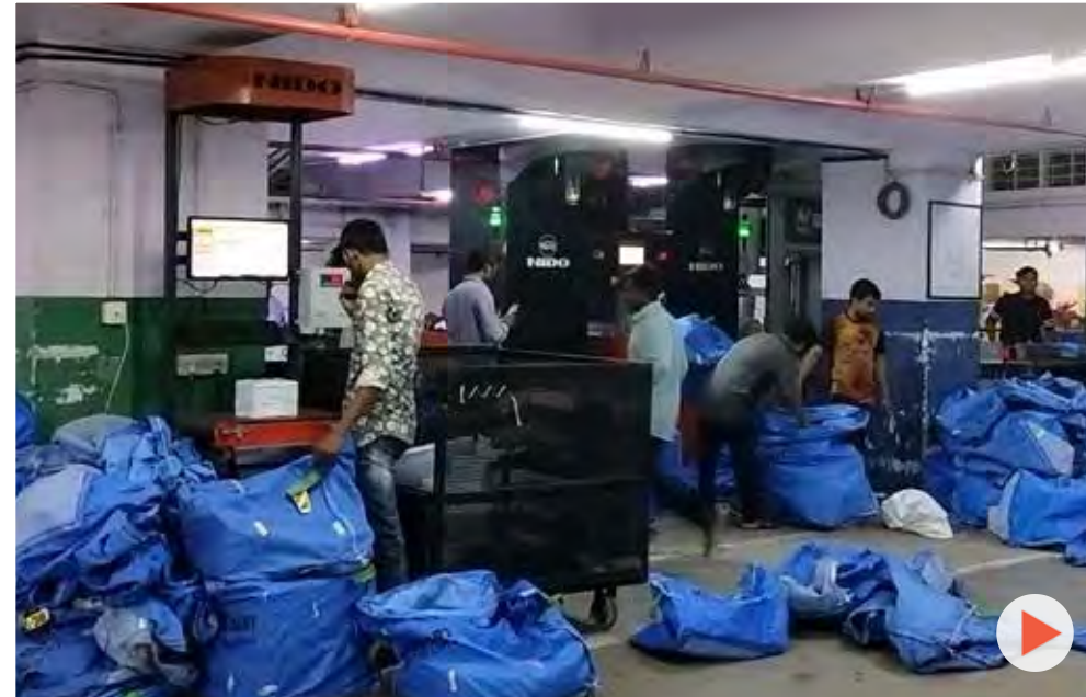
Camera based DWS System, Carriage belt sorter Scanning, weighing, dimensioning and sorting Industry: Courier express parcel
